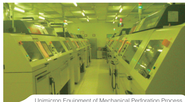
Unimicron Equipment of Mechanical Perforation Process
